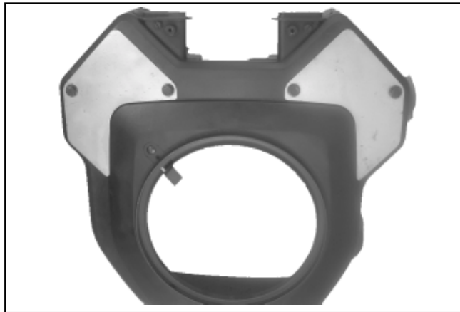
Figure 4-15. Cleanout Kit Installed on Blower Housing.
